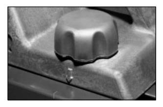
Loosen the lock knobs on the crossrail support by turning the knobs counterclockwise. Only loosen them enough to allow the crossrails to slide easily.
